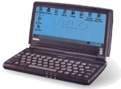
The touch-sensitive screen and a QWERTY-like keyboard provide input to the Palm-size PC. Some Windows CE-based handhelds and palmtops have a reduced size keyboard with the functionality of a full-sized keyboard. Other Palm-size PCs, specifically the smaller, palm-sized units use a software-controlled keyboard. The operating system displays a keyboard image on the display screen and the user taps each key to simulate an actual keystroke.
