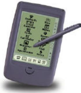
The Palm-size PC user interface supports a keyboard and stylus as input devices. The graphics engine provides support for color and grayscale display devices with up to 32 bits per pixel of color depth, palette management, TrueType and raster fonts, and advanced features such as shape drawing and bit block transfers. The graphics subsystem supports the full UNICODE standard, allowing Windows CE devices to be easily modified for non-United States markets.
