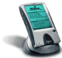
The Palm-size PC provides automatic, unattended synchronization of desktop and Palm-size PC data with the ActiveSync software. ActiveSync can synchronize any type of data with the desktop and the handheld PC. Companies that supply applications where data can be shared between the desktop and
